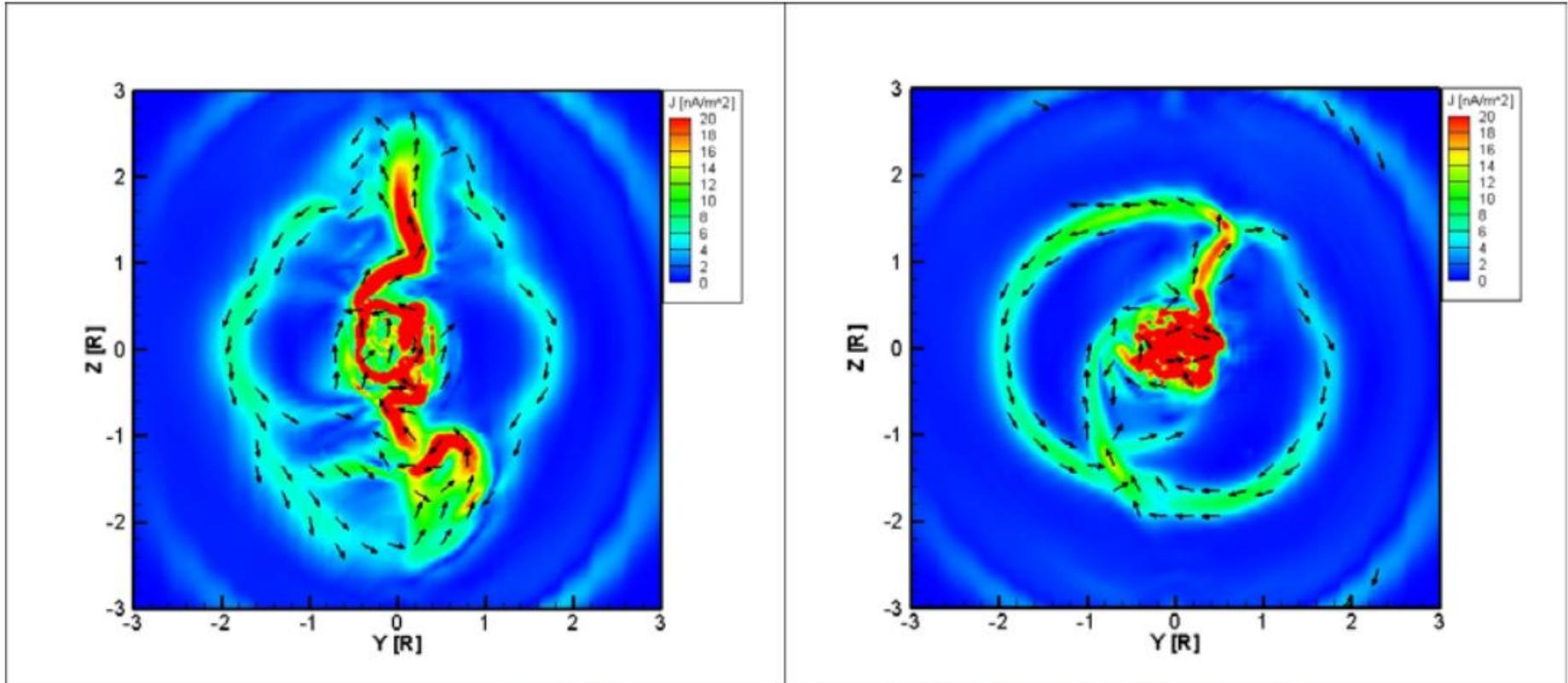
Slice of the current density vector at  $X = -1.1 R_M$ . Left: without crustal fields. Right: with crustal fields.
